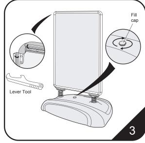
Use the lever tool to open the poster frame sides. Insert the poster behind the poster cover before closing the frame sides. Remove fill cap and use a hose to fill the base with water until overflowing. Alternatively sand can be poured in using a funnel.
