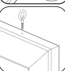
Screw eyes can be used for suspending this product. They can be positioned according to the below diagram.
