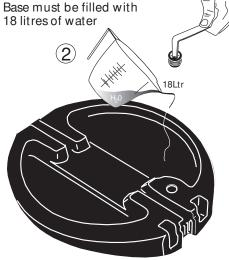
These cut outs in the base fit over the wheels on the frame
